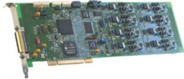
sertion is to ensure that the real-time simulator circuitry is not damaged. The PCI-RTA line of boards was designed with fault insertion in mind. Signal channels in each of the four PCI-RTA boards include hot short protection in +/-50V range and over-current protection.
