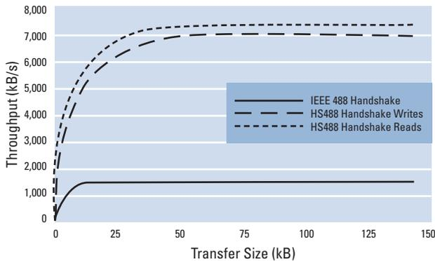
Figure 2. NI PCI/PXI GPIB Controller Data Transfer Benchmarks
