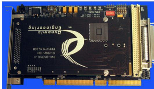
Front view of PCIBPMC with PMC\_BISERIAL II installed
