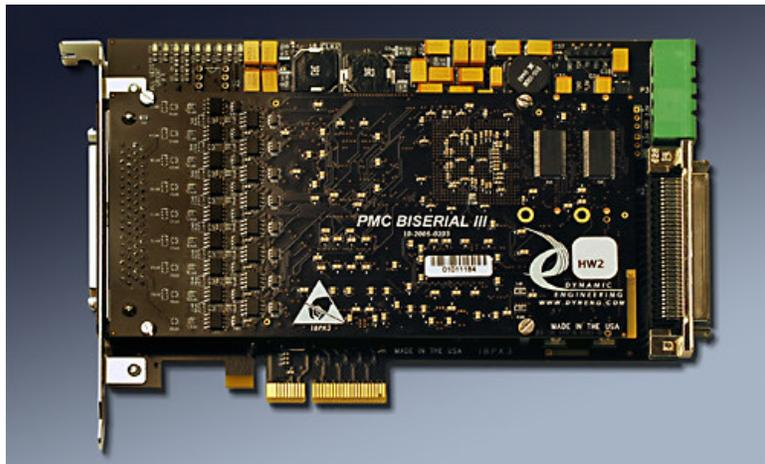
PCIeBPMC [X1 version] shown loaded with a Dynamic Engineering [PMC BiSerial III Module](#)
