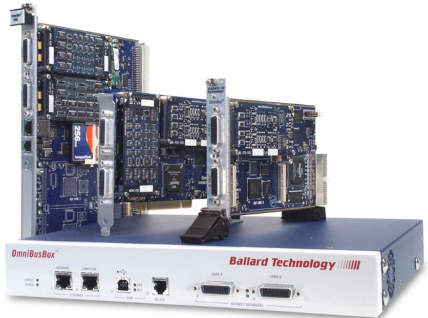
port equipment that varies from the ARINC 429 standard, such as some implementations of ARINC 575). ARINC 429 channels can be combined with ARINC 717 on the same module (see table of module part numbers on next page).
