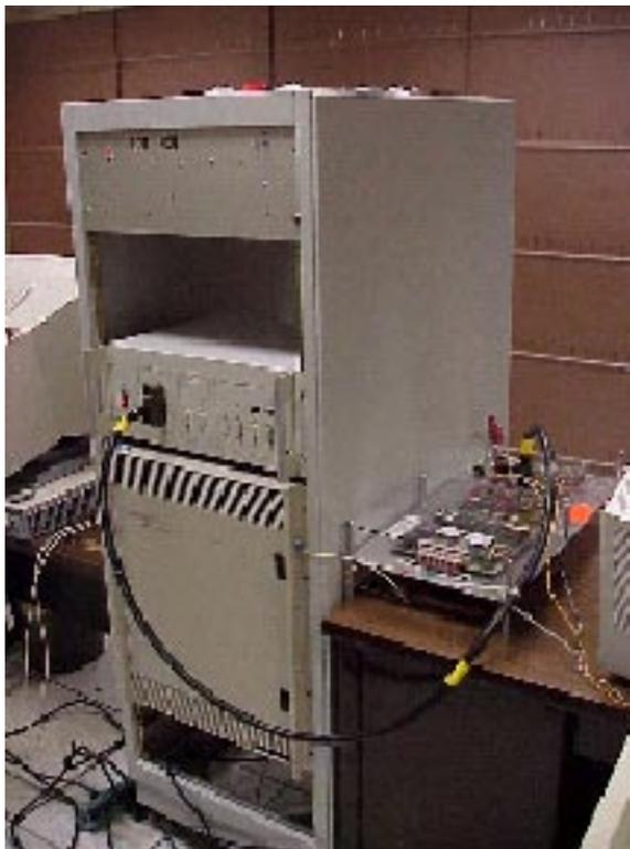
Development ECU breadboard connected to the RTS via the Simulation Interface Box. A flight ECU later replaced the breadboard.
